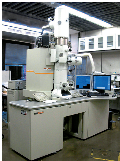
Figure 2. JEM-2100F, a TEM instrument used for the movie in Figure 1, is available in many institutions worldwide. A JEM-2100FC instrument equipped with an aberration corrector for the objective lens and a helium-temperature stage was used when necessary.
